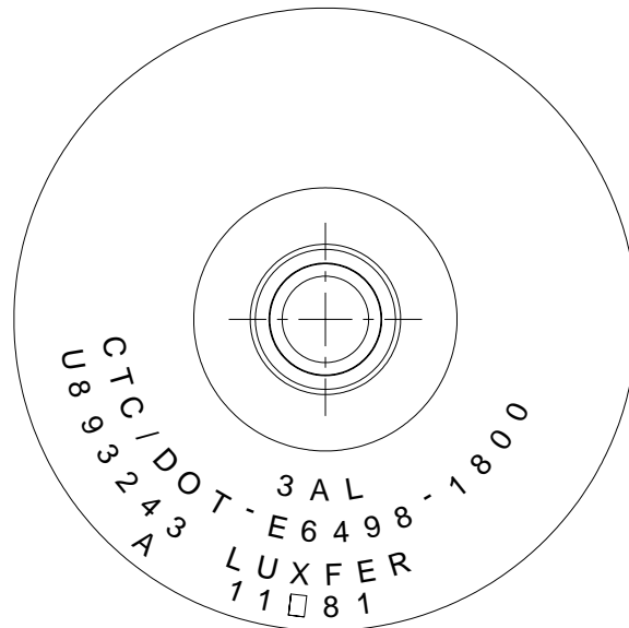
Figure 2—3AL marked exemption cylinder
